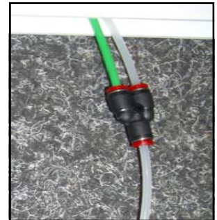
Bleed kit Y piece connected to pipes protruding from underneath skeg box
