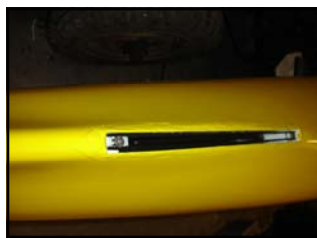
Gelcoat around finished skeg
