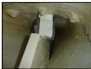
Skeg box wedged in hull with rubber blocks
