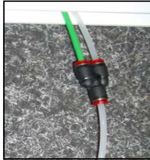
Bleed kit Y piece connected to pipes protruding from underneath skeg box
