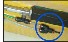
*Blanking plug by glide cylinder inside cockpit*
