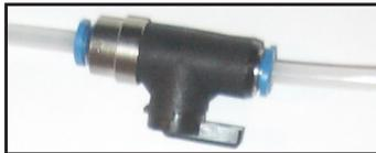
*Close-up of bypass valve, here shown in open position*
