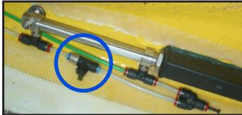
*Bypass valve and glide cylinder seen from inside the cockpit*
