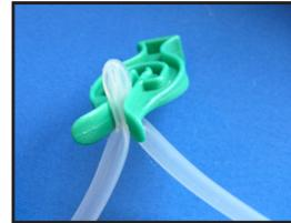
*Bleed kit pipe clamped shut with clothes peg*
