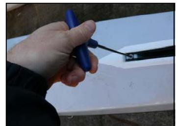
cleat assembly to the glide box with the screws provided (see below). Thread the 3mm cord through the glide tube and so out through the glide box, passing under the roller at the forward end of the box and back through the jam cleat as shown. Cut the cord to length and tie off the end to form a handle.
