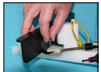
Connecting tiller block ram to operating pedal. This is best done with the block removed from the rail.
