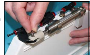
Attach actuator arm to rudder shaft crank arm.
