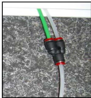
Bleed kit Y piece connected to tubes protruding from underneath skeg box
