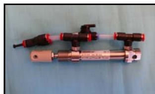
Rudder actuator ram assembly as supplied. The ram attaches to the top of the skeg box using the hole in the body of the ram, shown on the right in this image.
