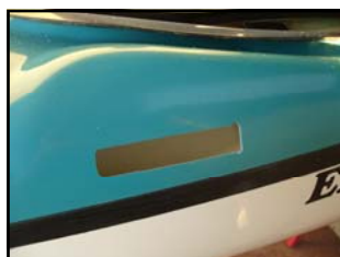
Glide box cut out on deck
