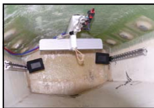
Example tiller block installation showing tiller pedal in relation to footpegs.
