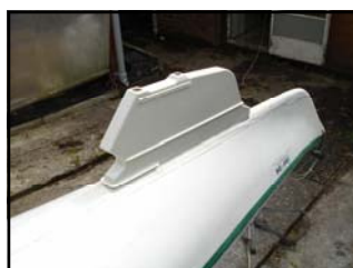
Skeg box positioned for marking out
