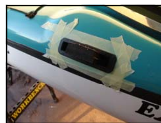
Glide box in place in deck
