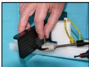
Connecting tiller block ram to operating pedal. This is best done with the block removed from the rail.
