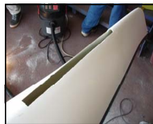
Skeg box cut out in hull
