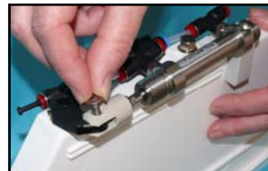
Attach actuator arm to rudder shaft crank arm.
