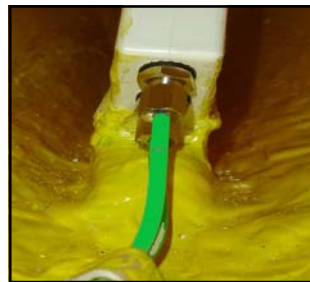
Green and clear tubes connected to skeg box
